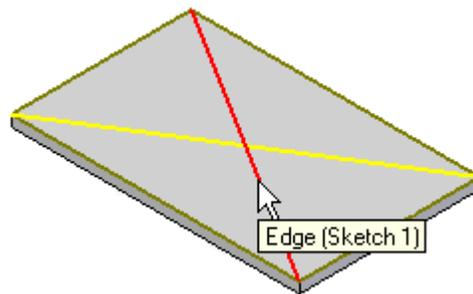
3. Specify the bend angle and direction for the cross brake.
