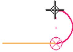
Place the arc end point vertical from arc start point.
