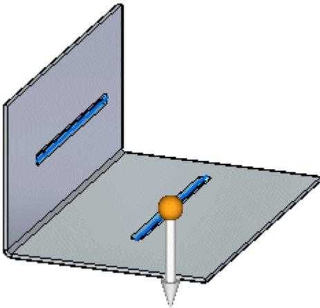
All disjoint beads created in a single operation offset to the same side.
