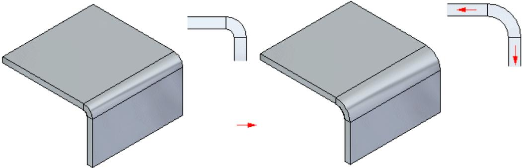
If you decrease the bend radius, the tab and flange extend into the bend to decrease the bend radius.
