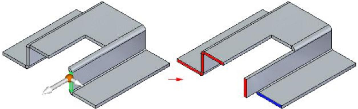
You may need to set the Orthogonal to Base if Possible option if you want to move or rotate a face that will cause a plate or thickness face to tip at an angle not orthogonal to the base reference plane.
