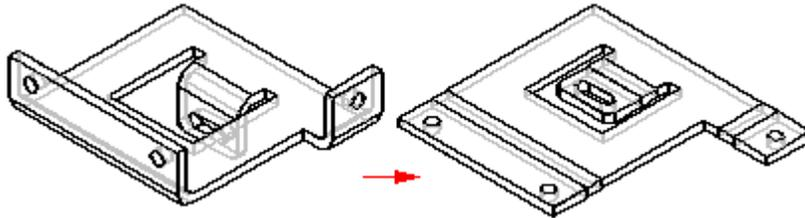
You can use the [Flat Pattern Treatments tab](#) on the Options dialog box to control output parameters for the flat pattern. For example, you can specify that any B-spline curves in the formed part are simplified to lines and arcs when creating the flat pattern. B-spline curves can be created when creating cutouts across bends and when using stencil font characters.
