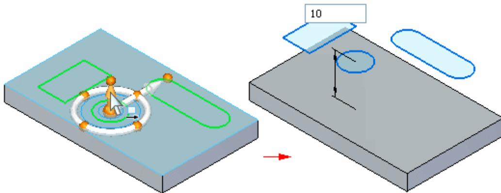
If the sketch is moved such that it becomes coplanar to another sketch, the two sketches are combined into one sketch, unless the Merge Coplanar sketches option has been cleared for one of the sketches.
