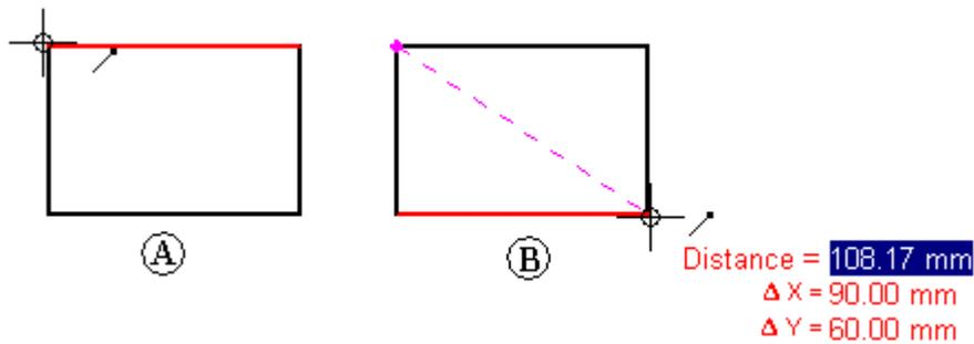
Clicking the keypoint adds it to a series of measurement points. Then you can select another point to see the new linear distance and deltas (C), or click it to see the distance between the last two points and the total cumulative distance from the origin to the last point (D). Click the right button to reset the command.
