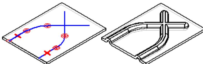
You can select more than one sketch element to construct multiple beads in a single operation.
