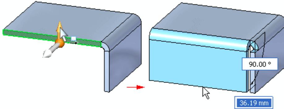
The flange start handle is also displayed without the 2D steering wheel when you click the Flange command on QuickBar when a planar thickness face is selected.
