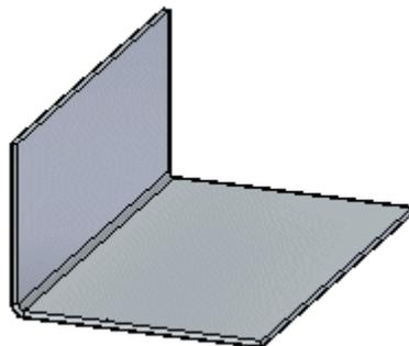
**Insert a bend in the synchronous environment with the Bend command**
