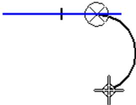
If you do not want the arc to be tangent to the line, you can move the cursor back into the intent zone region and out through the perpendicular zone before clicking to place the second end point of the arc.
