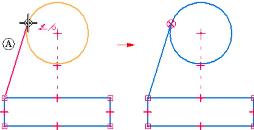
Until you click the point that completely defines the element that you are drawing, values in the command bar boxes update as you move the cursor. This gives you constant feedback on the size, shape, position, and other characteristics of the elements you draw.
