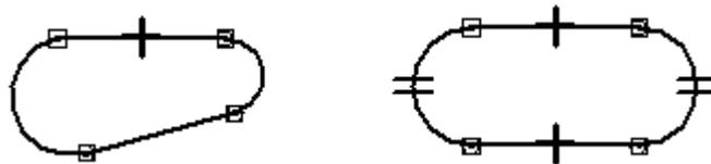
If a line and arc are not tangent (A), applying a tangent relationship modifies one or both elements to make them tangent (B).
