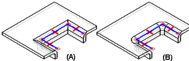
When you construct a drawn cutout, the sidewalls are constructed such that they lie inside the profile (A). After the feature is constructed, you can use the options to specify that the sidewalls lie outside the profile (B).
