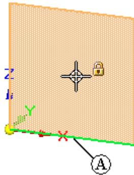
While you are defining the sketch plane and the default X-axis is highlighted (A), you can use the shortcut keys to change the X-axis orientation. For example, you can press the N key to select the next linear edge (B), or the B key to select the previous linear edge (C).
