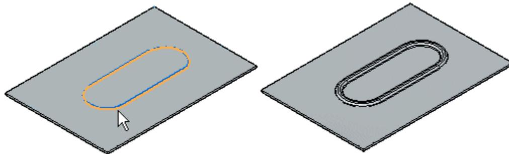
In the synchronous environment, you can construct a bead with an open sketch element,
