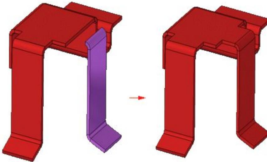
You cannot extend or trim manufactured features with the Attach command.
