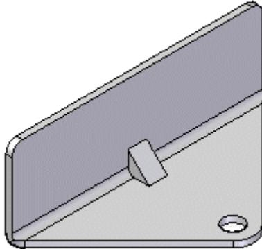
or, use the Pattern Type option to specify whether you want to place one gusset or a pattern of gussets. For example, you can use the Fit option to place three gussets that are equally spaced along the selected edge.
