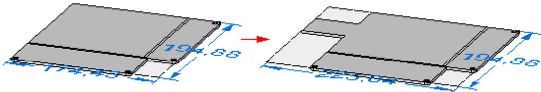
Any tabs created in the flat pattern are placed in the flat pattern node of PathFinder. Any material added to the flat pattern appears only in the flat pattern state. The folded model will not reflect the material addition.
