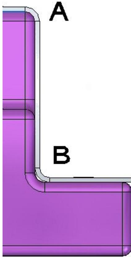
At (A) in the figure above, the sheet metal fits exactly over the 2.0 mm round on the part because the bend radius is 2.0 mm. The material thickness is 1.0 mm. The outer radius is the sum of these two values and is 3.0 mm. On the bottom bend, (B) the sheet metal does not fit exactly because of this. In the next step the bend radius will be modified so that the sheet metal part is correctly positioned at (B).
