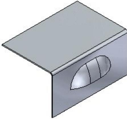
In the ordered environment, the profile for a louver feature must be a single linear element. Louvers cannot be flattened.
