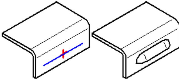
When constructing a louver, the louver height (H) must be equal to or less than the louver depth (D) minus the material thickness (T).
