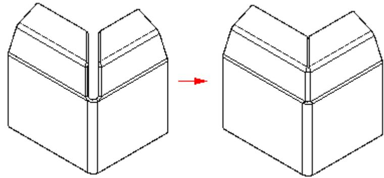
A closed corner is a treatment feature. You do not have to draw a profile, just select the edges you want to modify. With 2-bend corners, you can specify whether to close the corner (A), or overlap the corner (B).
