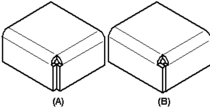
You cannot directly move or rotate a bend corner. However, you can move or rotate the bend corner by repositioning the adjacent flanges that form the corner. If a plate that contributes to the closed corner is deleted, the bend faces created by the closed corner are deleted and the closed corner definition is removed from the model.
