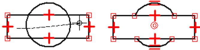
For example, you typically begin designing with key design parameters. You would draw known design elements in proper relation to one another (A) and then draw additional elements to fill in the blanks (B).
