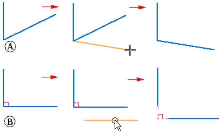
When you apply a relationship between elements, the relationship is maintained when you modify either element. For example:
