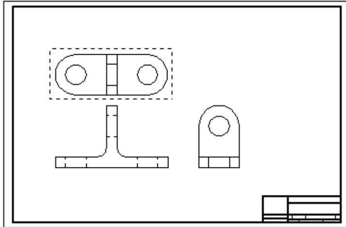
After you define all views, click the Finish button to launch the Part or Sheet Metal environment to create the model file in which the views are placed as sketches.
