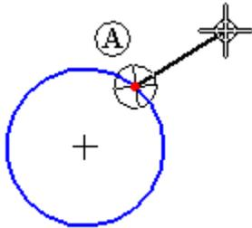
Two of these intent zones allow you to draw the line tangent to the circle. The other two intent zones allow you to draw the line perpendicular to, or at some other orientation relative to the circle.
