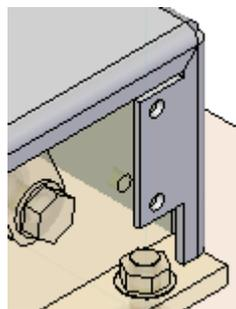
**Step 9:** The tab and holes on the sheet metal part need to be adjusted to lie on the mounting face of brake assembly. Use the Jog command to accomplish this.
