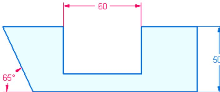
To change a dimension value of a locked dimension, click the dimension value and enter a new value.
