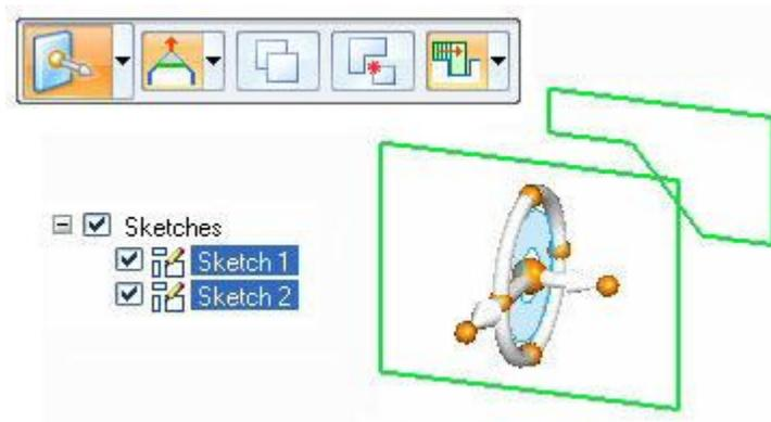
Use the secondary axis or handle plane to move sketch elements in a plane.
