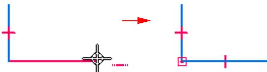
Relationship handles displayed on the 2D geometry show you how elements are related. You can remove any relationship by deleting its handle. You can display or hide the relationship handles with the Relationship Handles command.
