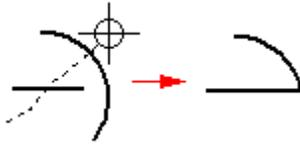
The Extend to Next command extends an open element to the next element. To do this, select the element and then click the mouse near the end to extend.
