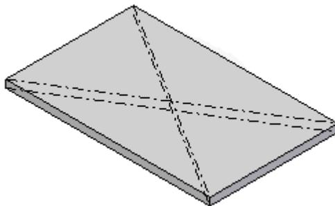
A cross brake feature does not deform the 3D model. It adds attributes containing information about the bends. This attribute information is used when creating a flat pattern or drawing of the sheet metal part.
