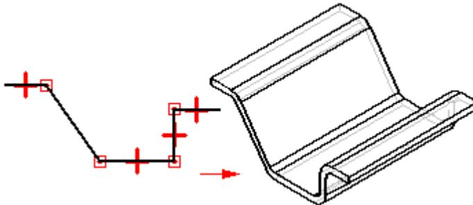
The Lofted Flange command quickly constructs a flange using two open profiles on parallel reference planes. Like the Contour Flange command, the Lofted Flange command automatically adds bends using the bend radius property. You do not have to draw an arc at each bend location.
