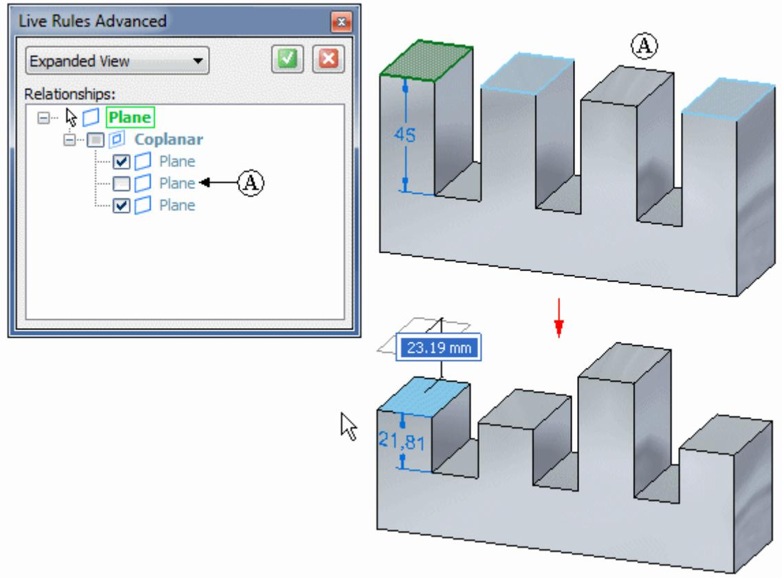
You can also clear the check box adjacent to the relationship heading (A) to specify you do not want any of the deselected coplanar faces to remain coplanar when you move the selected face.
