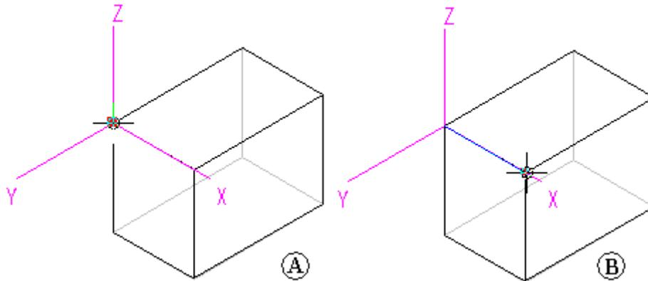
In the Part, Sheet Metal, and Assembly environments, the Measure Angle command measures angles. You can measure between any two faces or between any three points.
