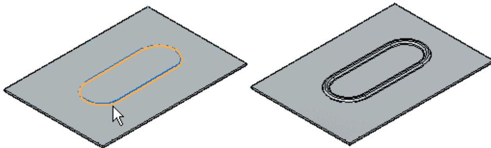
When constructing a bead profile using multiple elements, the element must be a continuous set of tangent elements.
