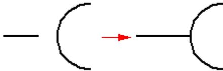
You can also select an element to extend to. This selection overrides the default option of extending to the next element only. To select an element to extend to, press the Ctrl key while selecting the element to extend to. For example, in normal operations, if you selected line (A) as the element to be extended, it would be extended to the intersection of the next element (B). However, you can select edge (C) to extend the line to that edge.
