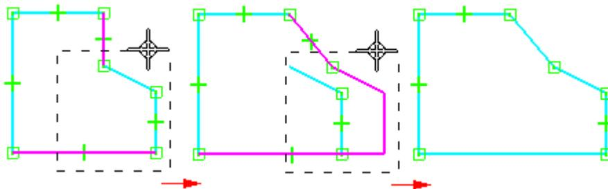
Relationships are added or removed as necessary during element modification. If you trim part of a circle and more than one arc remains, concentric and equal relationships are applied between the remaining arcs.
