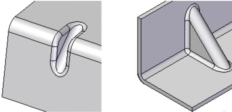
You can create a gusset automatically or from a user-drawn profile. You can use the Gusset Options dialog box to specify the method to use when constructing the gusset. The steps required to construct the gusset are different depending on the method you use.
