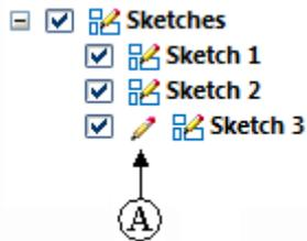
If there are existing sketches in the model, you can lock and unlock the sketch plane using the Lock Sketch Plane command on the PathFinder shortcut menu when your cursor is over a sketch entry.
