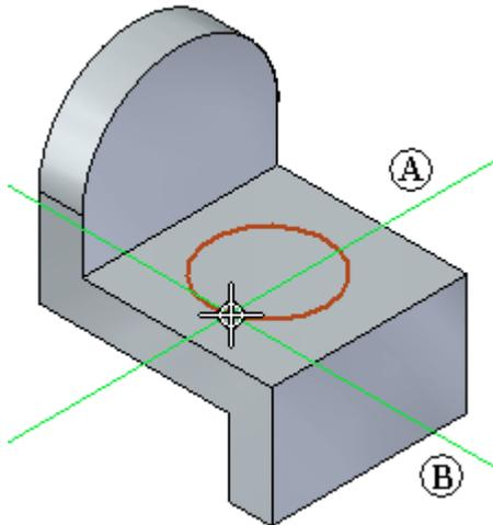
The sketch plane remains locked until you right-click to restart the current command, or start another locked command. This ensures all sketch input lies on the current sketch plane.
