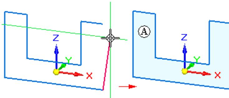
In a part or sheet metal document, you can use sketch regions to construct features using the Select tool. Sketch regions are formed automatically when a series of sketch elements close on themselves (A), or when sketch elements and one or more model edges form a closed area (B).
