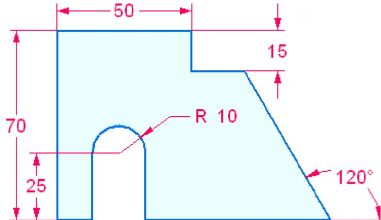
2D sketch geometry defines the cross-sectional shape used to create a base solid body or the shape used to create a feature on an existing solid body. Sketches are drawn in 3D on either a planar face or a reference plane. You lock onto a planar face or reference plane to draw sketch geometry.
