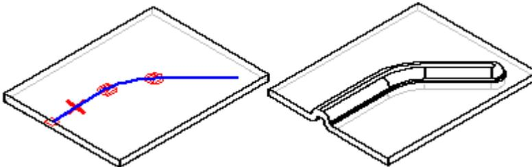
You can also construct a bead feature using multiple, separate sketch elements. Each element must be a continuous set of tangent elements, but the profiles can cross each other.
