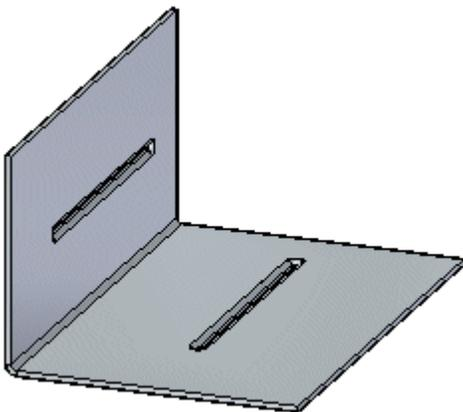
When constructing multiple disjoint beads, an entry in PathFinder, a feature profile, and a nail is created for each disjoint bead. Beads cannot be flattened and they cannot cross a bend.
