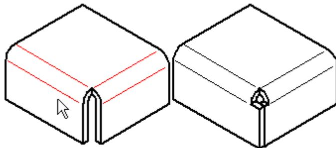
In the ordered environment, when you overlap a corner, you can use the Overlap Ratio option to compute the overlap as a percentage of the global material thickness.
