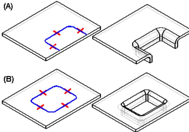
The ends of an open profile must theoretically intersect a part edge. A closed profile cannot touch any part edges. A drawn cutout can be constructed only on a planar face. You can use the Drawn Cutout Options dialog box to specify punch radius, die radius, and taper options.
