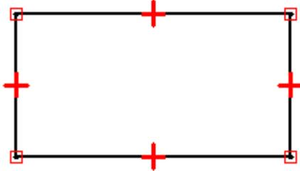
You can also use the Connect command to connect the endpoint of an element to any point on another element, not necessarily an endpoint or keypoint. This is called a point-on-element connection, and the symbol resembles an X. For example, the endpoint of the top horizontal line on the right side of the profile is connected to the vertical line, but not at an endpoint.
