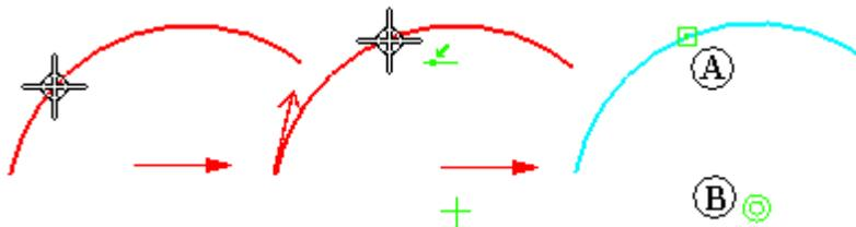
Fillet and Chamfer commands combine drawing and trimming operations.
