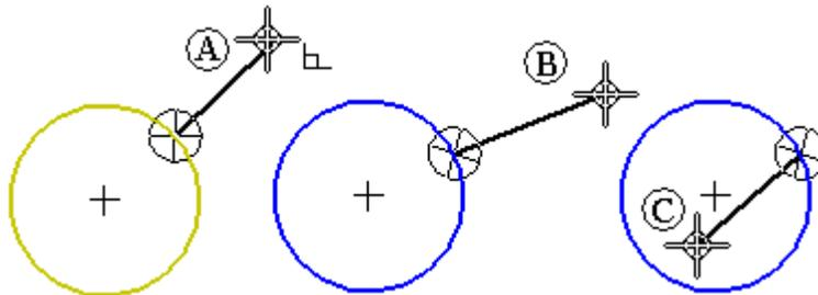
The Line command also allows you to draw a connected series of lines and arcs. You can use the L and A keys on the keyboard to switch from line mode to arc mode. When you switch modes, intent zones (A) and (B) are displayed at the last click point.
