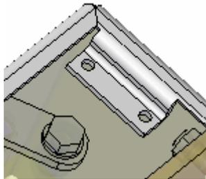
**Step 10:** Remove the sharp corners on the jog tab.
