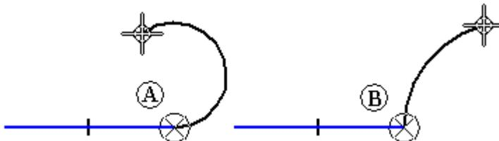
The intent zones allow you to control whether the new element is tangent to, perpendicular to, or at some other orientation to the previous element.
