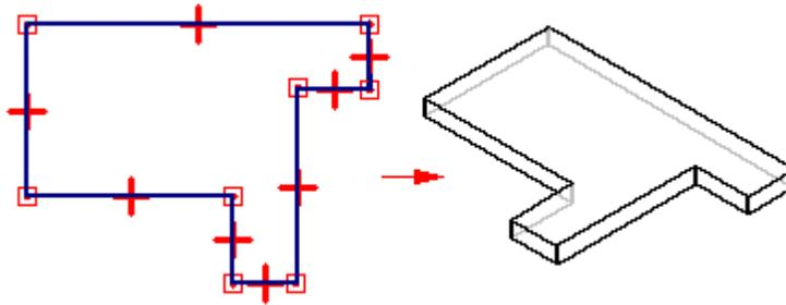
The **Contour Flange** command constructs a feature comprised of one or more bends and flats using an open profile.
