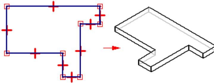
For subsequent features in the ordered environment, the profile can be open or closed. When using an open profile, you must define the side of the profile to which you want to add material.
