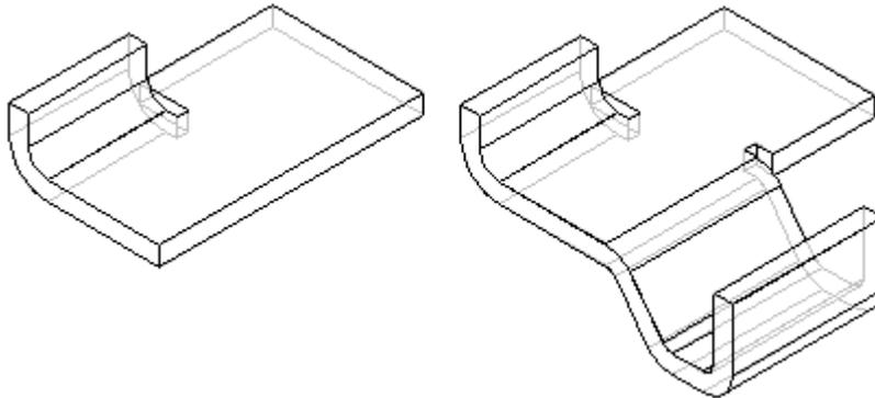
You could do this by selecting the endpoint of the edge shown to locate the new reference plane, and then clicking the face shown on the right side of the figure to define the base of the reference plane.
