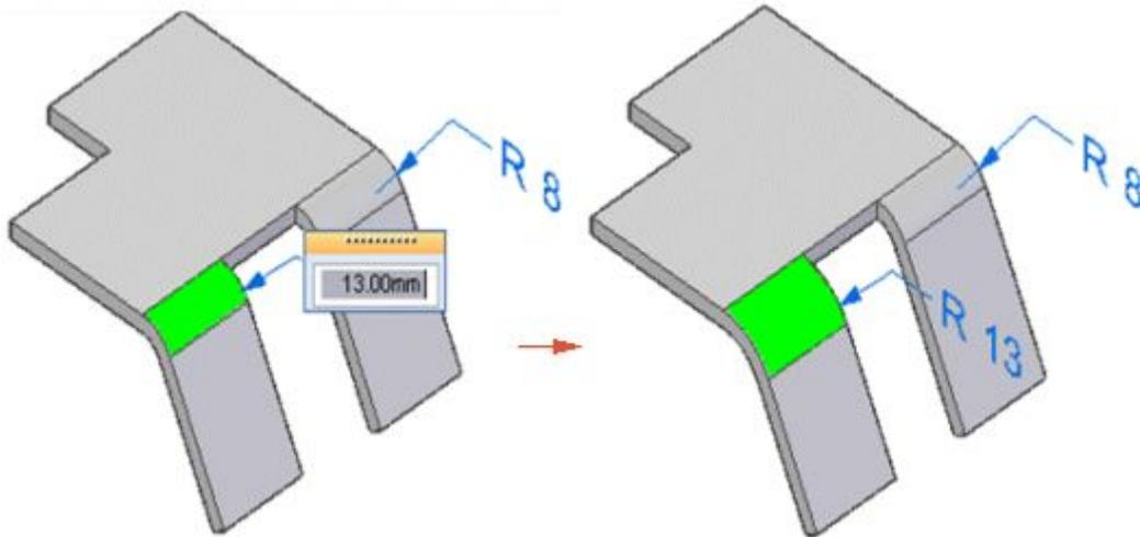
If the split bends were originally a single bend in a flange, and then cut to make two separate flanges,
