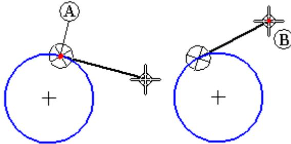
If you do not want the line to be tangent to the circle, you can move the cursor back into the intent zone region and out through one of the perpendicular zones (A) before clicking to place the second end point of the line. When you move the cursor through the perpendicular zones, you can also draw the line such that it is not perpendicular to the circle (B) and (C).
