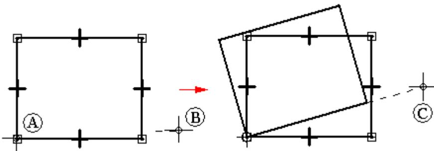
The Scale command uses a scale factor to proportionally scale or scale and copy 2D elements.
