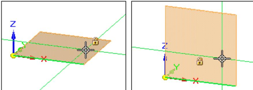
When you click to define the first endpoint of an element, such as a line, sketch input is locked to the current plane.
