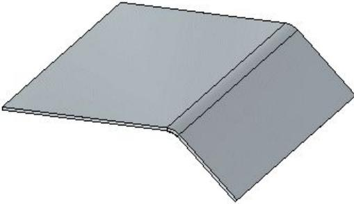
If you increase the bend radius, bend relief is applied to the model and the bend extends into the flange.
