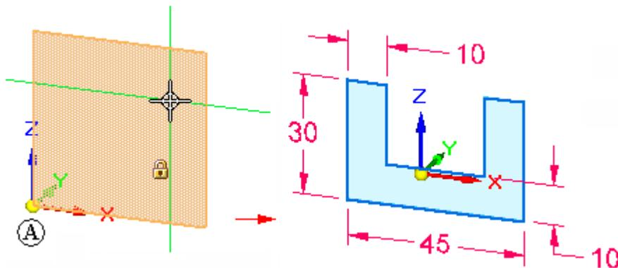
You can see which plane of the coordinate system you will draw on because the plane under the cursor highlights, and the alignment lines, which extend out from the cursor, adjust dynamically depending on what plane your cursor is over.
