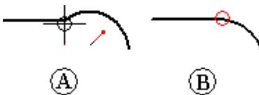
When you use relationship commands, the software allows you to select only elements that are valid input for that command. For example, when you use the Concentric command, the command allows you to select only circles, arcs, and ellipses.
