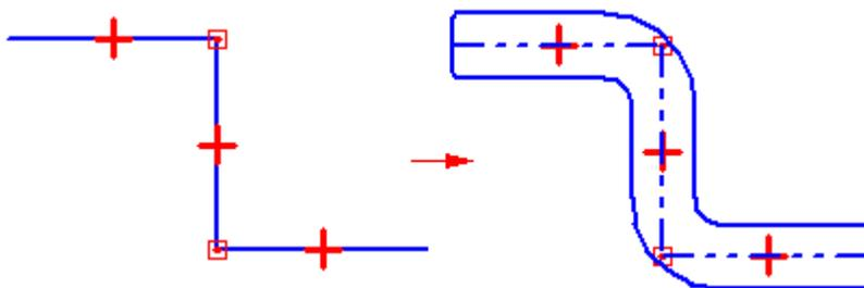
The Stretch command moves elements within the fence and stretches elements that overlap the fence.
