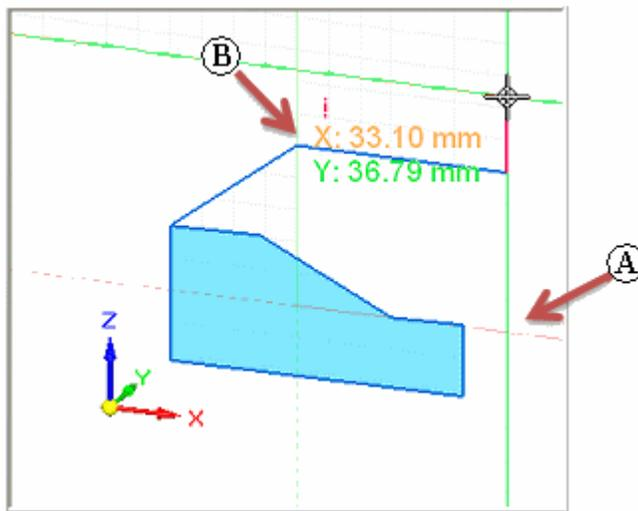
If the Snap To Grid option is on when you add dimensions and annotations, they will snap to grid lines and points.
