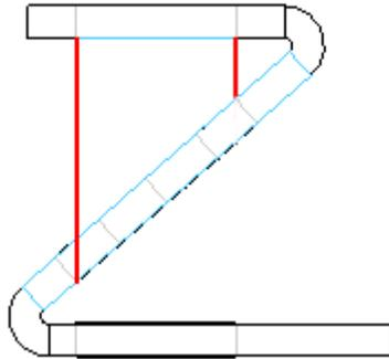
The Thickness cut option is useful when creating parts in which a shaft must pass through aligned circular cutouts.
