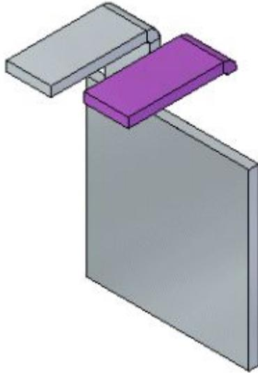
When the flange is attached to the main body, all other required faces are automatically created.
