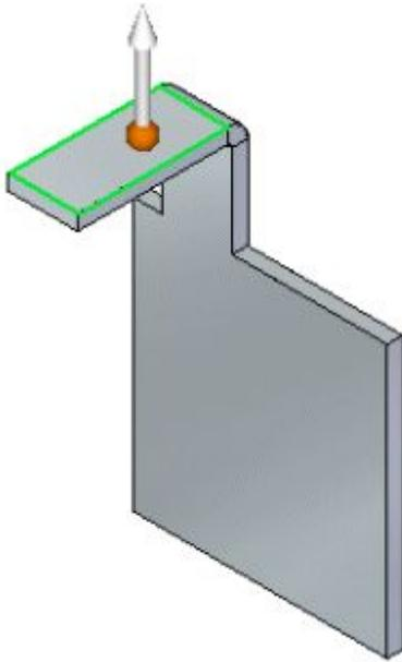
Once you copy the flange and then select the Paste command, a glass image of the flange attaches to the steering wheel.
