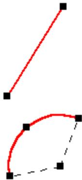
You can change the shape of a selected element by dragging one of its handles. The first figure shows the effect of dragging an end point handle. The second figure shows the effect of dragging the midpoint handle.
