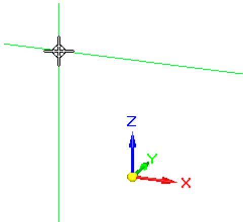
Notice the alignment lines connected to the cursor. These lines assist you in aligning sketch geometry.
