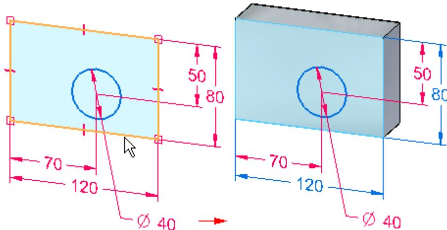
During this process, dimensions and constraints may be connected to both body edges and to remaining sketch geometry. If the sketch contains stacked dimensions, then some dimensions in the stack may migrate individually. Other dimensions, such as coordinate dimensions, do not migrate until all of the 2D geometry they are attached to has been used to construct a feature.
