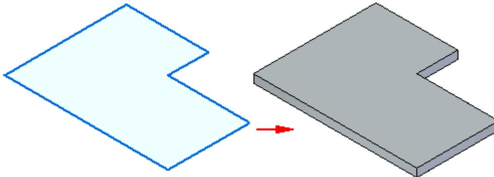
For subsequent features in the synchronous environment, the sketch can be open or closed. If the sketch is open the edge of the tab must close the sketch to form a sketch region. Subsequent features are automatically added when you select the extrude handle.
