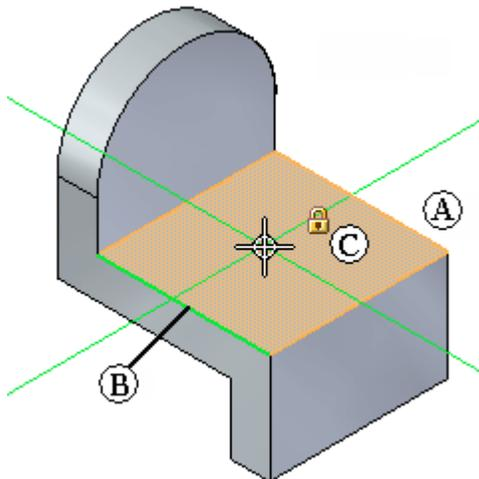
When you click to position the starting point for the sketch element, the sketch plane is automatically locked to the highlighted plane or face. The alignment lines (A) (B) remain displayed as you draw to indicate the current sketch plane's X and Y axes.
