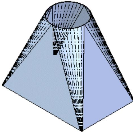
You can set the number of bends. For the lofted flange to flatten, the arc angle must match between the two cross sections.
