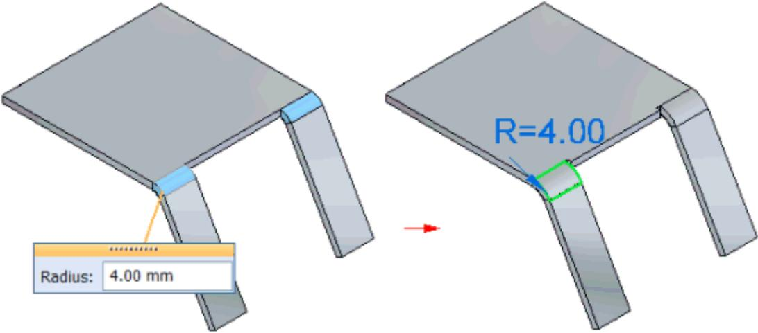
If the flanges on both sides of the bend are bound by the model, the bend radius for each bend row is edited together. For example, if you edit the radius for the top bend, the radius is updated for the top bend in both flanges.
