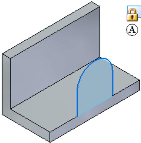
When you want to unlock the sketch plane, you can click the locked plane indicator symbol in the graphics window to unlock the plane, or you can press the F3 key.
