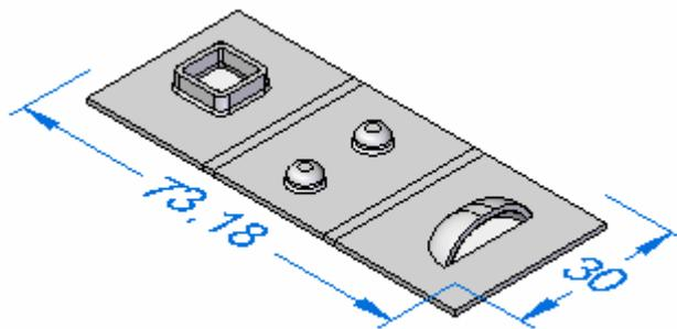
**As Feature Loops**    Displays the sheet metal features as feature loops in the flat pattern.
