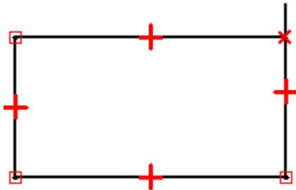
When drawing profiles, pay close attention to the relationship indicator symbols that IntelliSketch displays, and try to draw the elements as accurately as possible. Otherwise, you may accidentally apply a connect relationship in the wrong location, which can result in an invalid profile. For example, for a base feature you may accidentally create an open profile, rather than the required closed profile.
