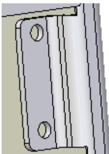
**Step 11:** The cover is a symmetric part. Mirror the features to the other side of the part.
