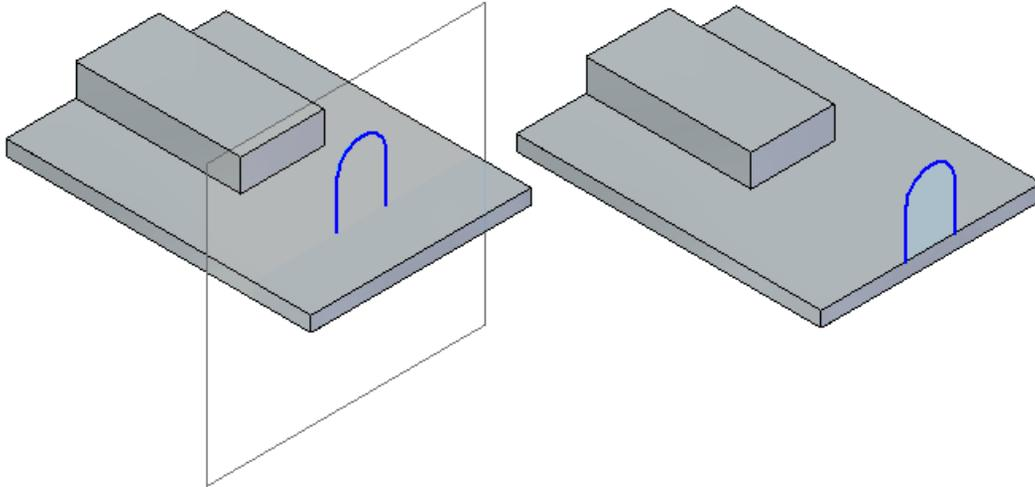
An open sketch that is not coplanar with a body face or is coplanar with a body face but does not touch or cross a face edge does not create a region. A region is created if an open sketch is connected to or crosses a coplanar face edge.
