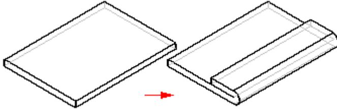
In the ordered environment, you can construct a hem along any edge on a sheet metal part. For example, you can construct a hem along a linear edge
