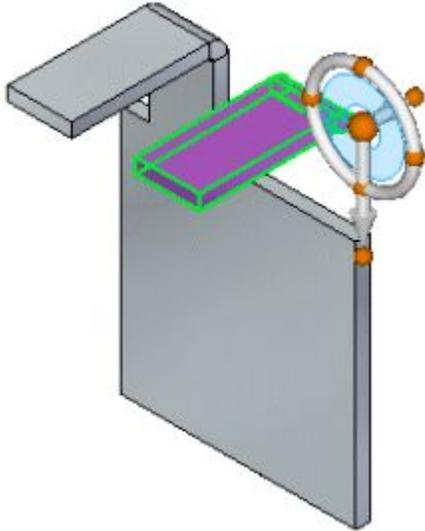
You can locate and lock to a plane and then use the steering wheel to adjust the position of the detached flange.
