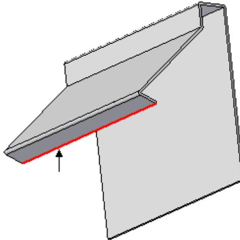
Type 20 mm in the Distance field and set the direction as shown.
