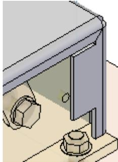
**Step 8:**    Insert two holes in the tab to line up with the holes in brake assembly.
