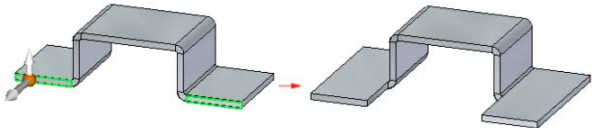
Selecting the Suspend Live Rules option does not affect the setting of the Thickness Chain option. In other words, if the Thickness Chain option is set and you select the Suspend Live Rules option, the Thickness Chain options remains set.
