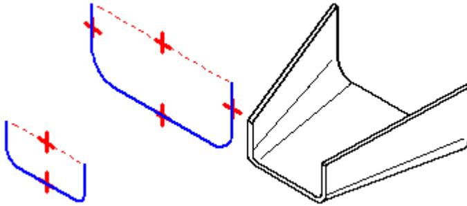
The Bending Method tab on the Lofted Flange dialog box creates incremental bends for all bends in the flange.
