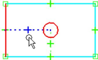
This can be useful when multiple relationships are in the same location and you need to delete one relationship. In this situation, you can use QuickPick to highlight the relationship, and the parent elements are displayed using a dashed line style.
