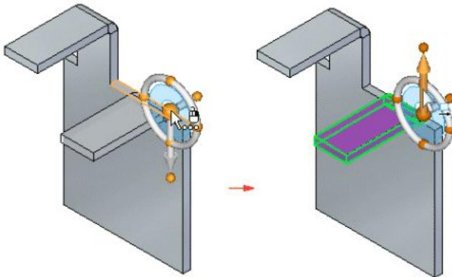
Once the position of the flange is valid so that it can be attached, you can use the Attach command to attach the flange to the main body of the model.
