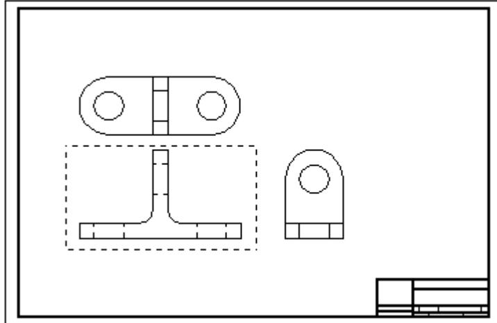
If you select the Fold Principal Views option or Fold Auxiliary Views option and it is not the primary view, you can click the Fold Line button after you select all of the elements for the view. The Fold Line button allows you to define a line or point in an orthogonal or auxiliary view on which to fold the primary view.
