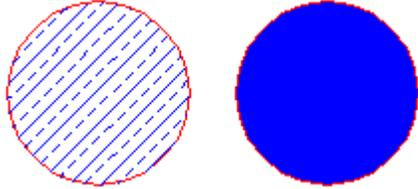
A fill is like other elements in that you can format it and move it around, but the fill is always associated with a boundary. The boundary can be made up of more than one element.
