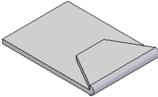
A positive value will miter the flange outward and will typically add material.
