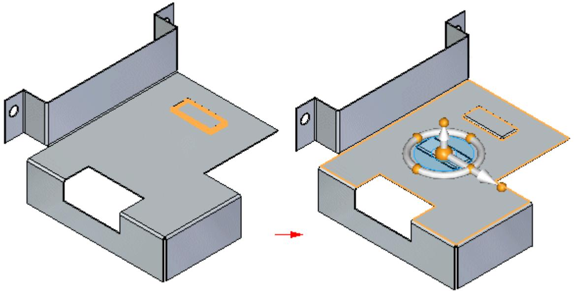
Once you have pasted the feature, you can use the Attach command to attach the feature to the face.
