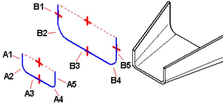
If the two profiles have the same number and type of elements, and each element on the first profile maps to the same element type on the second profile (line to line, or arc to arc), in most cases, you can flatten it.
