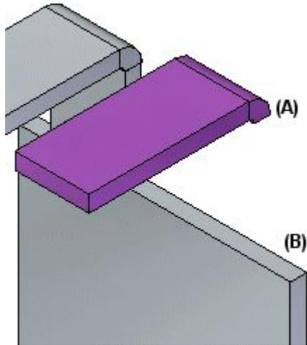
The flange bend can also be embedded into the boundary of the plate.
