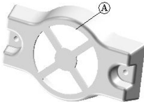
Each of the four cutouts must sweep 90°. A narrow web of material must occupy space between each cutout to avoid breakout. To create this model, use construction elements to locate the cutout, provide the mechanism for the sweep angle, and provide the distance between each cutout.
