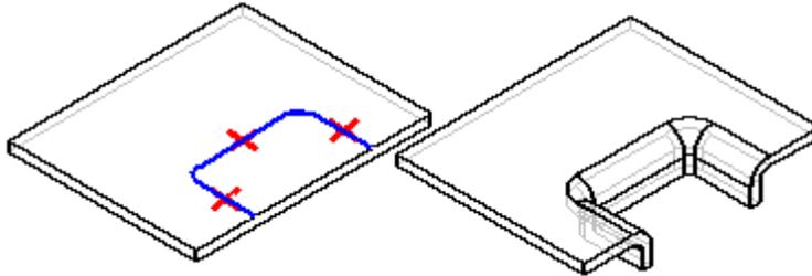
In the synchronous environment, the geometry used to create the cutout can be a closed internal profile that creates a region or an open profile extended to a part edge to create a closed region.
