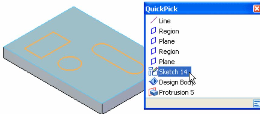
You can then use the steering wheel to move or rotate the sketch to a new position in space.
