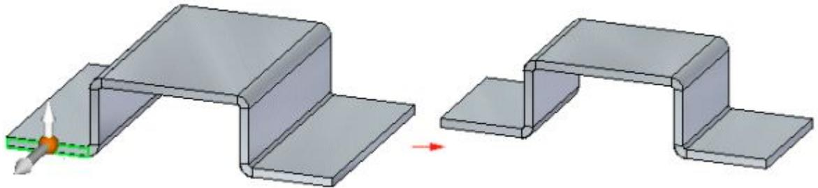
When the Thickness Chain option is not set, only the selected face or faces move.
