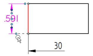
In this ISO dimension, the terminator handle was used to display a half dimension rather than a full dimension. The dashed lines show the dimension line and the projection line that were turned off.
