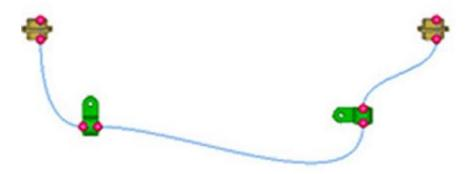
When you set the fixed length, a free edit point is added at the midpoint (1) of the longest segment between edit points on the curve.
