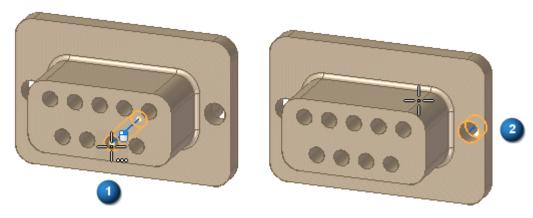
If you select the option, you can locate the center point (1) because it has an assigned terminal. However, you cannot select the cylindrical face (2) because it has no assigned terminal.
