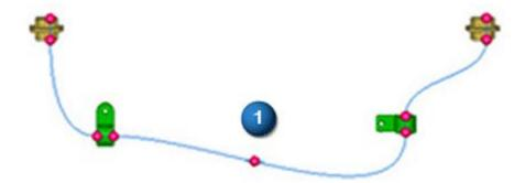
• You can use the end point of an existing path (1) to create a new path (2) that is tangent and continuous to the original path.
